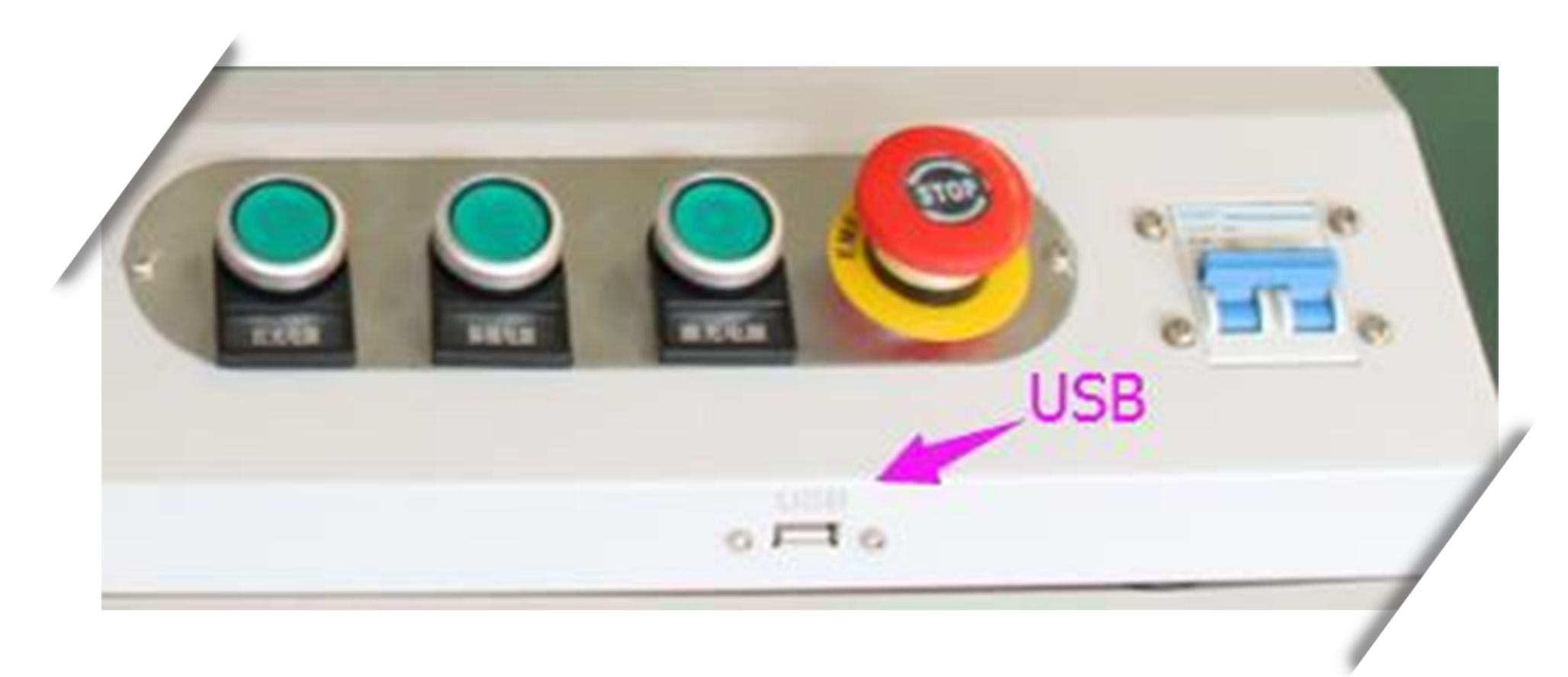
USB line, connect the control cabinet and computer, as in the above pictures.
